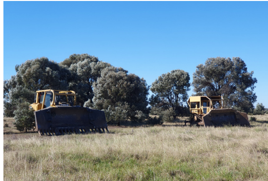
Dozers about to commence Brigalow scrub pulling and raking in Meandarra, QLD Source: Herron Todd White
